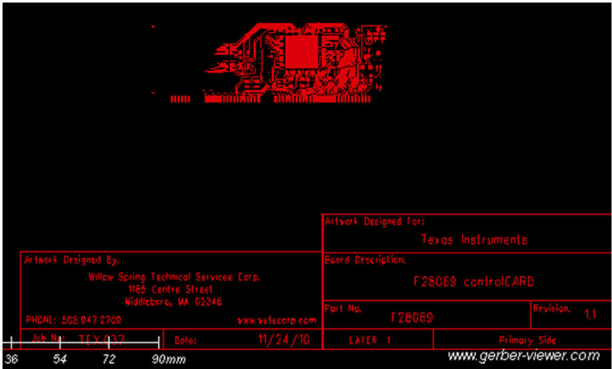
Figure F6.2B – Gerber Photoplot
